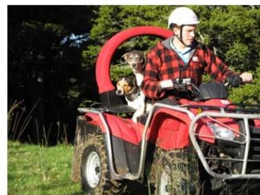
Although used for these purposes, there is continuing evidence of death and serious injury when quads are used for spraying, carrying or towing loads. These activities reduce the stability of quads, leading to an increased likelihood of death or injury from crashes and rollover.
