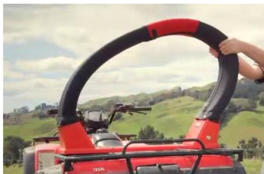
Figure 3. TRAX LifeGuard CPD system, showing deformable characteristics [14].
