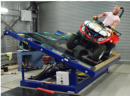
Figure 10. ATV tilt table static stability test being carried out at Crashlab, UNSW-TARS project, Feb 2013. Quad Bike loaded with rider (95<sup>th</sup> % Hybrid III ATD, with front load and rear Quadbar CPD fitted.
