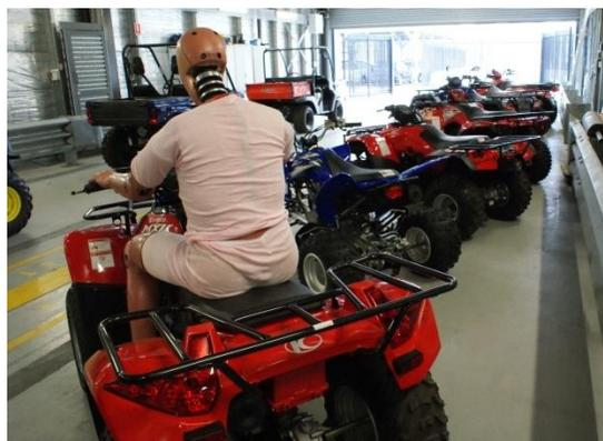
Figure 7 One of the "workplace" Quad Bikes at Crashlab, with a Hybrid III ATD 'rider', and other Quad Bikes and SSVs at Crashlab.
