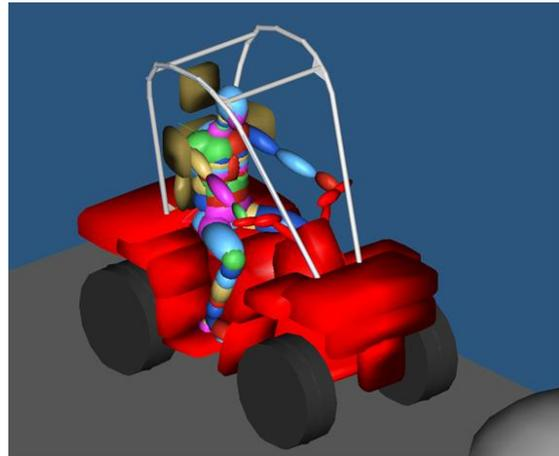
Figure 1. Proposed MUARC ROPS for ATV, with four-point seatbelt; winged seats. MADYMO model analysis.
