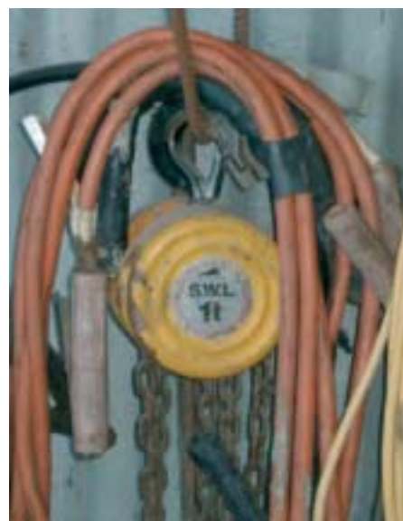
Clearly visible safe working limit
