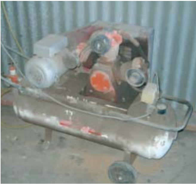
An air compressor with the appropriate belt guard
